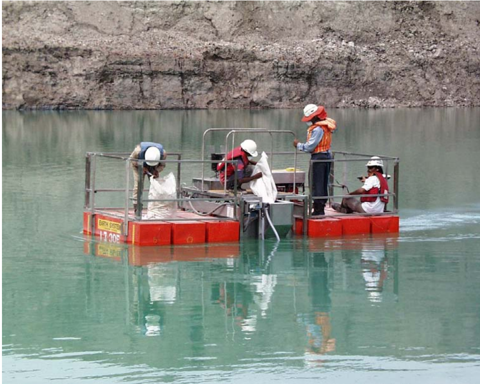
Figure 2: Treating Turbid Water Using The Portable Neutra-Mill (During Training).
