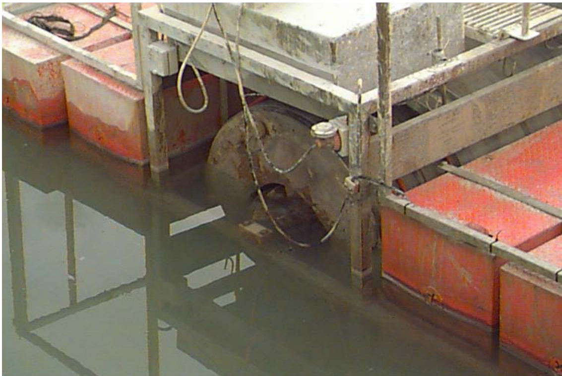
Figure 1. A Portable Neutra-Mill Showing the Partially Submerged Drum
