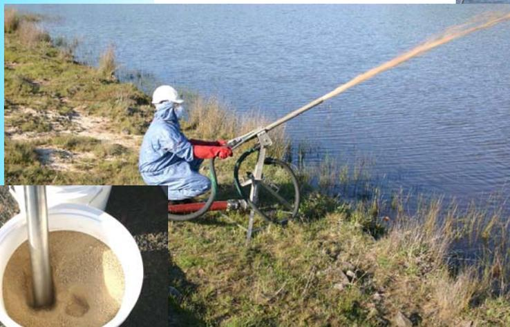
Shore based dispensing with Hydro Slurry System
