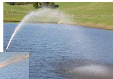
Hydro Slurry spraying over water– the system is capable of distributing a plume up to 20 metres from shore
