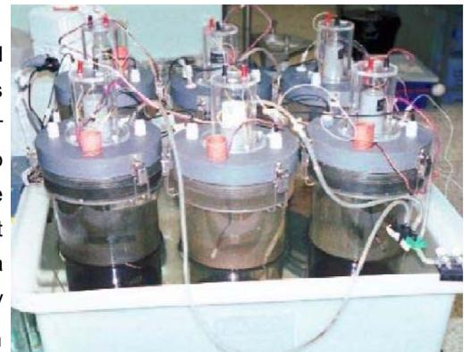
*Laboratory testing of nutrient release from sediment cores*
