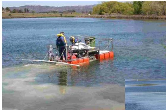
Pond being treated using a floating Neutra-Mill
