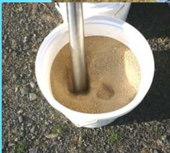
Dry powdered reagent being vacuum fed from a small stockpile
