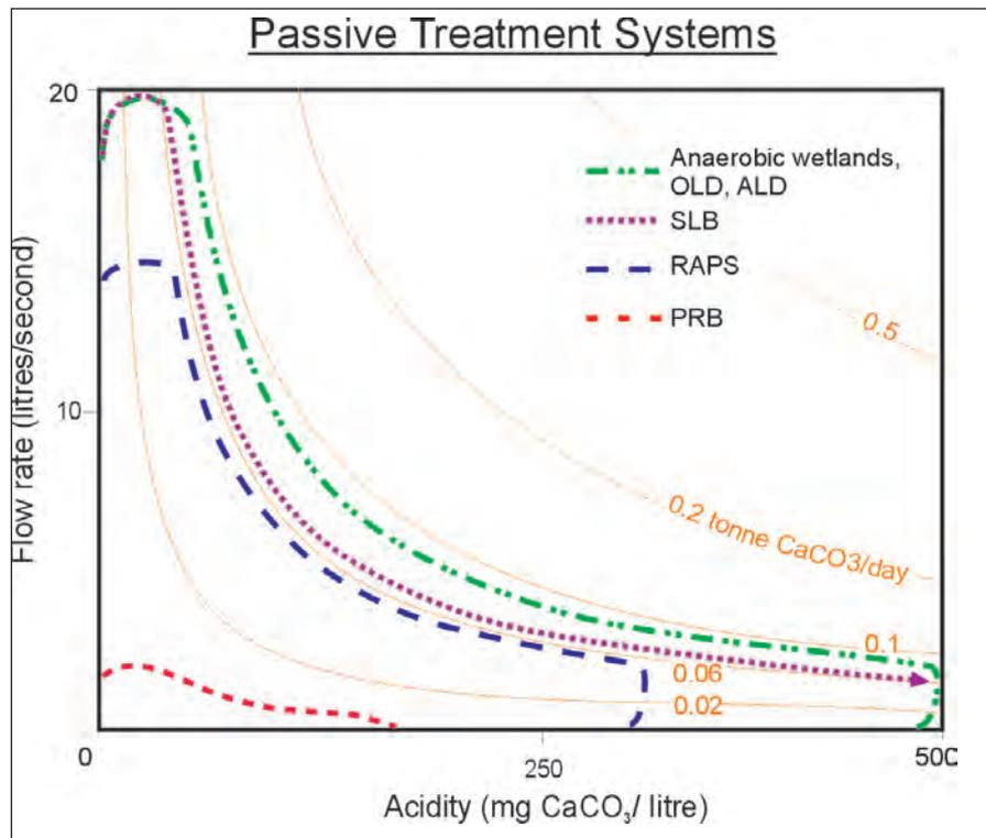
installed in inappropriate situations. They can be constructed to channel flows or implemented within existing drainage lines. OLDs are best suited to treat ARD with pHs above 2, acidities below 500 mg CaCO<sub>3</sub>/litre, flow rates of less than 20 litres/s, and total acid loads less than 150 kg CaCO<sub>3</sub>/d (see Figure 2).
