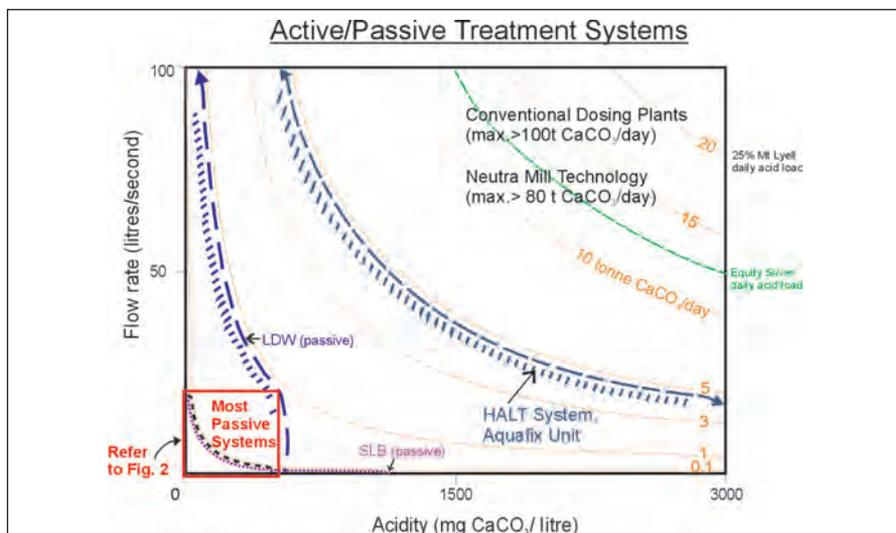
used in isolation, passive treatment systems have proven to be most successful at addressing post closure ARD issues, particularly at some coal mines. It is critical that they be deployed within their chemical and physical limitations. While passive treatment systems have always been regarded as providing lower cost solutions, the inappropriate application of such
