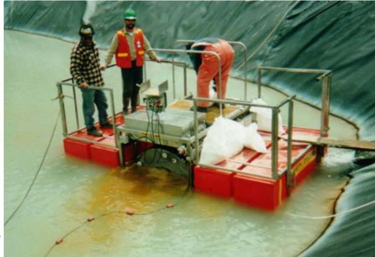
dosing units. These dosing units are based on the patented, Neutra-mill technology, and are capable of dispensing up to 5 tonnes of dry powdered reagent per hour.
