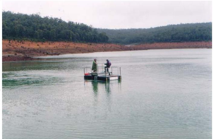
**Water-based mill used for emergency turbidity control in a drinking water storage reservoir.**
