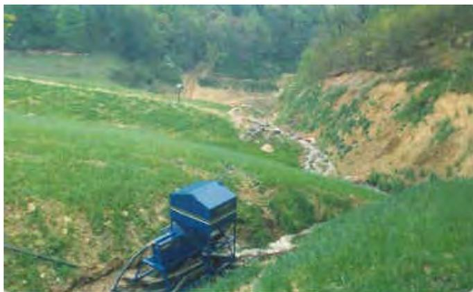
Plate 14. Aqua-fix system treating AMD from a waste rock pile.
