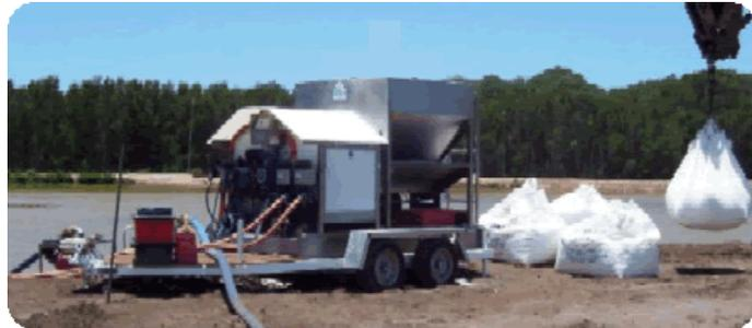
Plate 13. Calibrated Reagent Applying Blender (CRAB) system.
