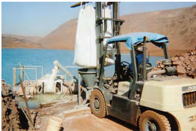
Plates 11-12. The Neutra-Mill can be used for in-situ (active) treatment of large open water bodies, such as pit lakes, or streams affected by AMD. The equipment can be water-based (above) or land-based (right), and does not require manual operation.
