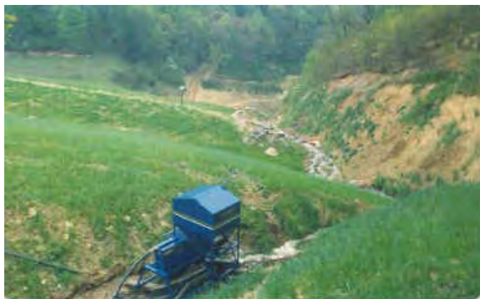
Plate 14. Aqua-fix system treating AMD from a waste rock pile.
