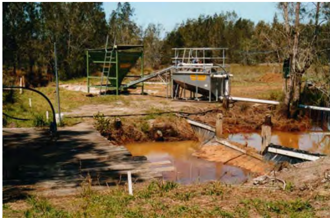
Plate 15. This portable land-based HALT mill can be used for in-situ (active) treatment of large open water bodies, such as pit lakes, or streams affected by AMD.
